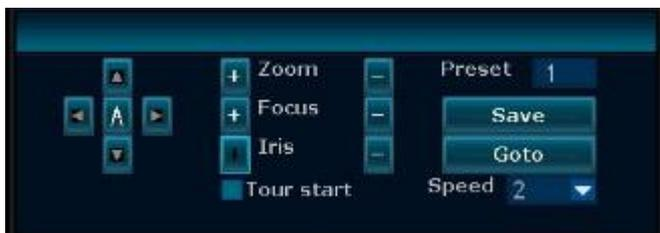
*Note: xmartO PT(WP1324) camera only supports Pan & Tilt. You can click the Up, Down, Right and Left button to make the camera pan and tilt.*
