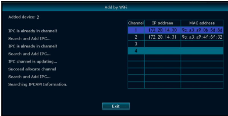
If you see message “IPC is already in channel!”, it means the camera has been added to the NVR successfully. You can then click “Exit” to leave the interface. In Device Manage interface, you will see the camera with IP address 172.20.14.xx show up in bottom box. As shown in below picture:
